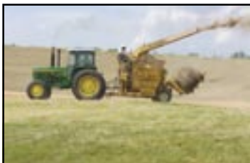
Turfing erosion control.
